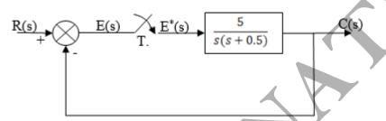
Figure Q6. Sampled data controller
