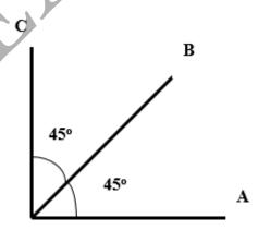
Figure Q5 45<sup>0</sup> rectangular strain gauge rosette
