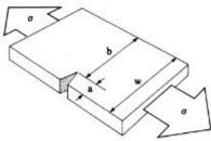
(4) Edge crack of length a in a plate of width w.
