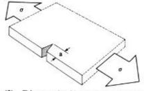
(2) Edge crack of length a in an infinite plate Y = 1.12 Because plane strain and plane stress have
