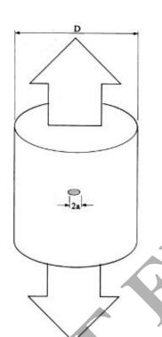
(5) Penny-shaped internal crack of radius a.
