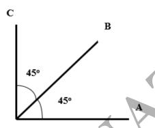
Figure Q5 45<sup>0</sup> rectangular strain gauge rosette
