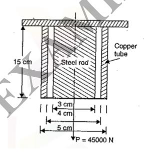
Figure Q5a. A Compound bar
