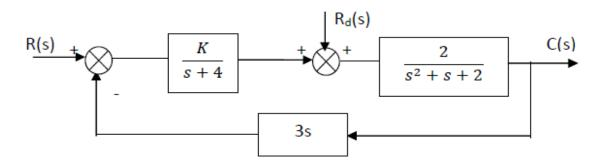
Figure Q6 - A position control system
