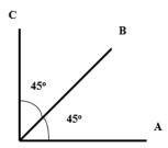
Figure Q5 45<sup>0</sup> rectangular strain gauge rosette
