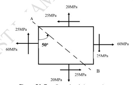
Figure Q3. Two dimensional stress system
