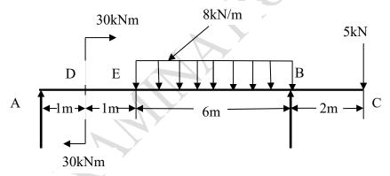
Figure Q1 simply supported overhanging beam
