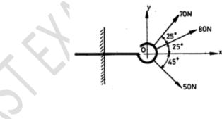
Figure Q5b. Forces on a hook
