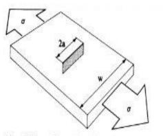
(3) Through crack of length 2a in a plate of width w.
