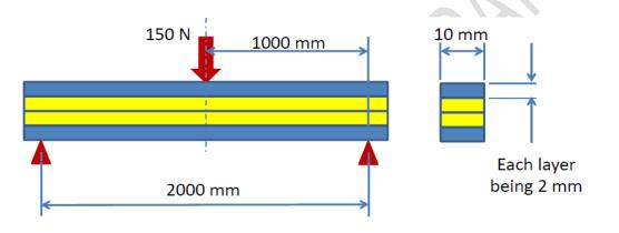
Unidirectional glass reinforced polymer (UD – GRP)
