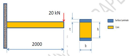
Figure 2: Composite sandwich panel with cross section.
