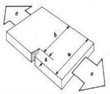
(4) Edge crack of length a in a plate of width w.
