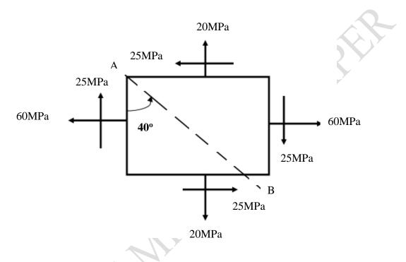
Figure Q3. Two dimensional stress system
