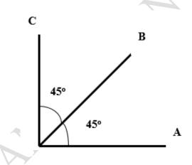
Figure Q5 45° rectangular strain gauge rosette
