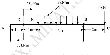
Figure Q1 simply supported overhanging beam
